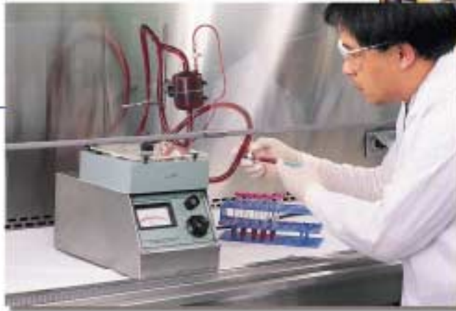
Left: Sample aliquots are removed from a simulated cardiopulmonary bypass circuit. Right: SLS scientist examines sub-micron contaminants captured on membrane surface.
